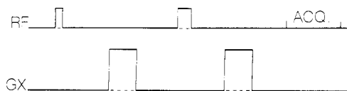
Figure 4. The timing diagram for the pulsed gradient spin-echo pulse sequence for determining self-diffusion coefficients.
